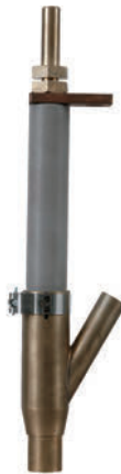
OBT 1200 043900 1,200 amps at 100 percent duty cycle. For 1/16–5/32 inch (1.6–4.0 mm) wire. Torch has concentric flux flow nozzle and features a replaceable breakaway adapter end to prevent costly damage should torch run into an obstruction.
