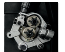
Heavy-duty aluminum two-drive-roll system
